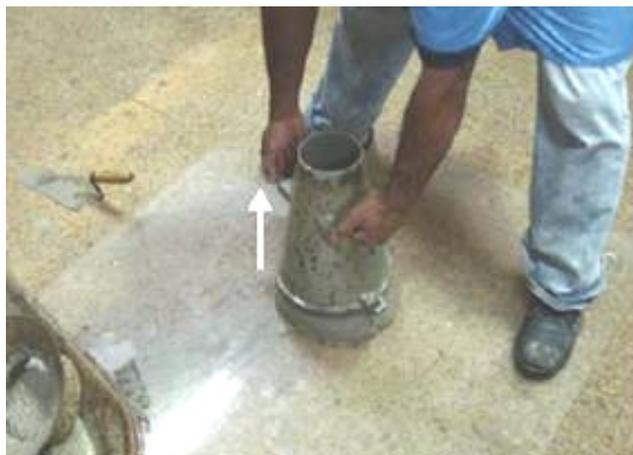
Figura 2.12 – Slump Test (LIMA, 2006)
