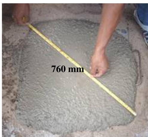
(a) *Slump Flow Test*
