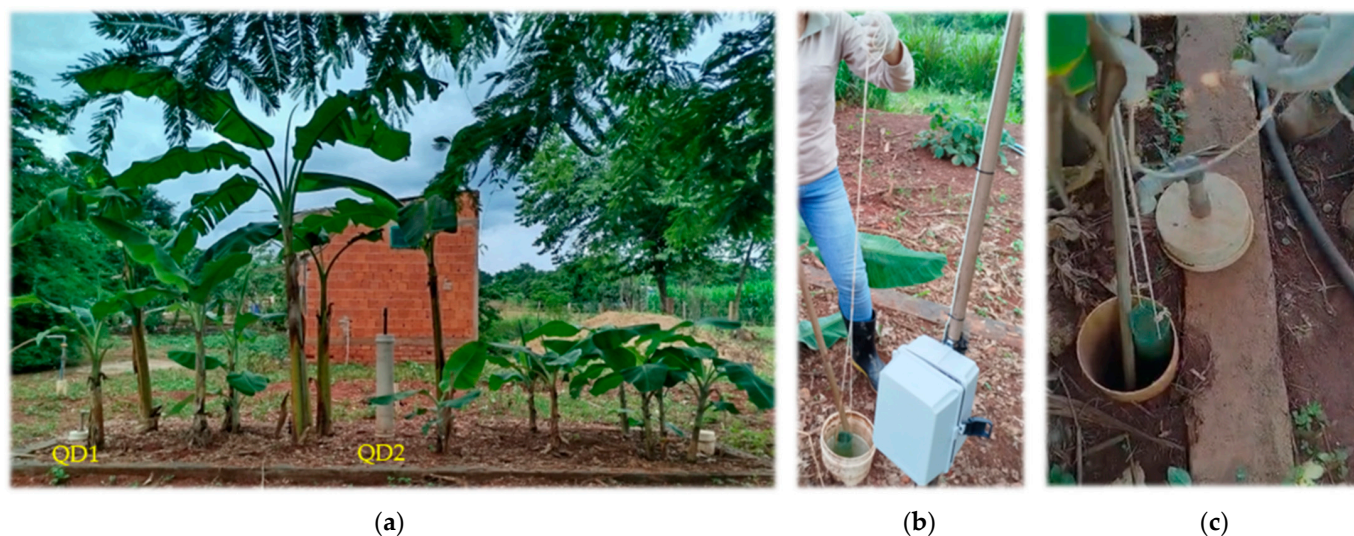
Figure 4. Collection of blackwater samples inside the TEvap at two different points (a): inlet (QD1) and midpoint of the system (QD2), using a manual sampler (b) made from a plastic bottle (c).
