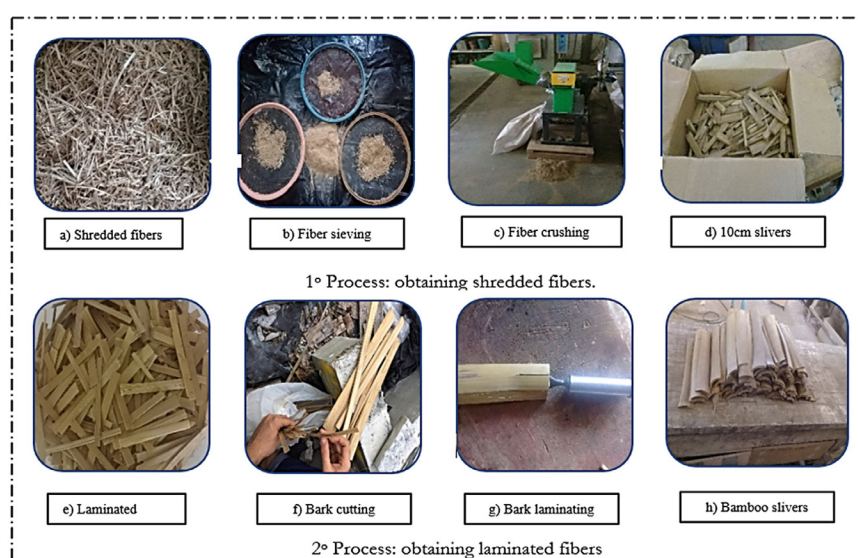
FIGURE 2. Process for obtaining bamboo fibers: the 1 st process from a) to d) with crushed fibers and the 2 nd process from e) to h) with laminated fibers.
