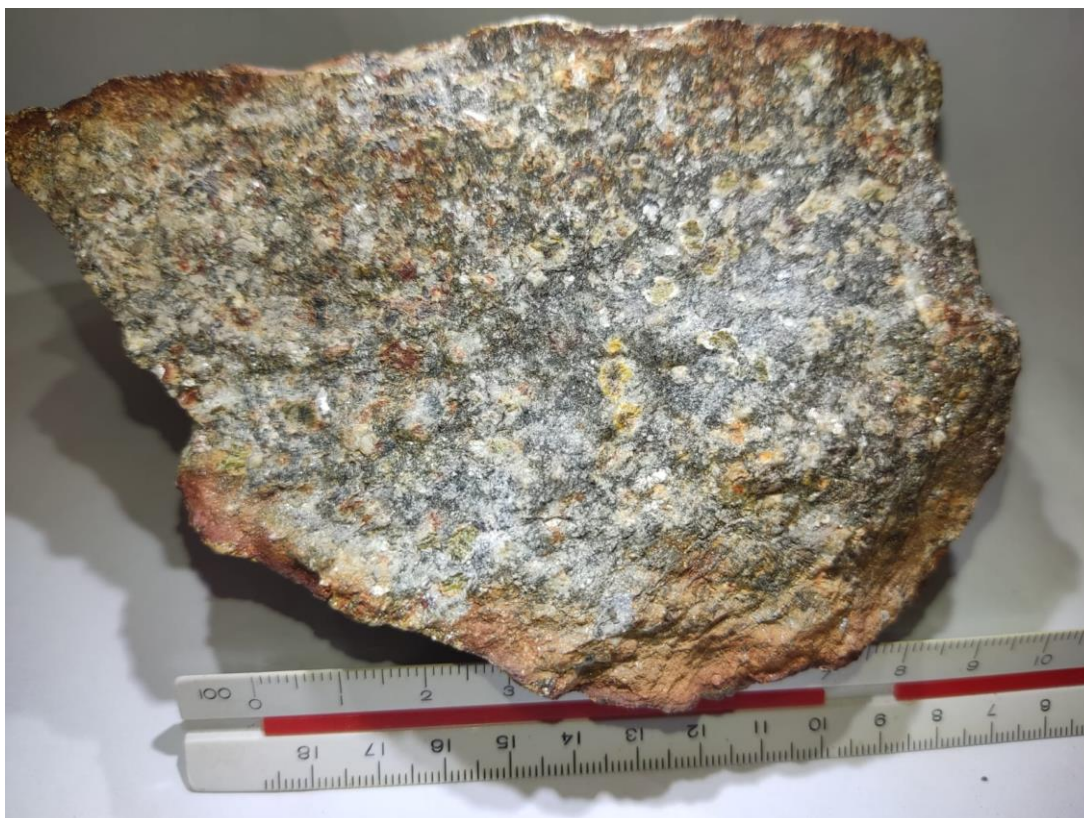
Figura 24: Amostra magnetita-coríndon-muscovita granofels. Ponto 22TF01_74 UTM 620758; 8171089.
