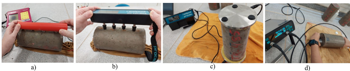
Figure 5: The non-destructive tests used: (a) and (b) surface resistivity tests, (c) bulk resistivity test and (d) ultrasonic pulse velocity test.
