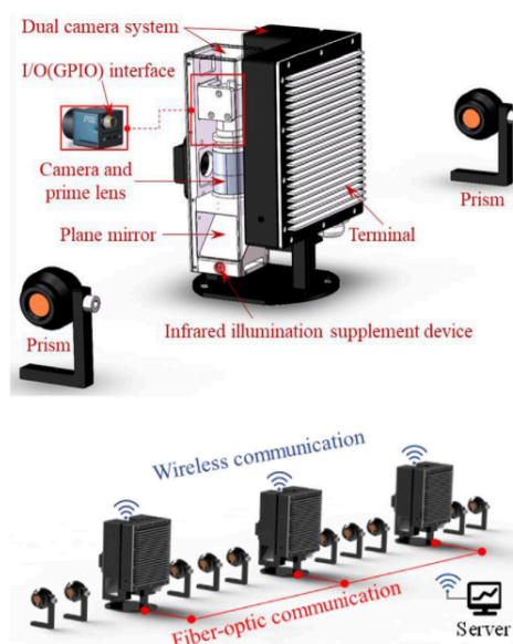
FIGURE 2 Camera network system (CNS) of bridge deflection monitoring.
