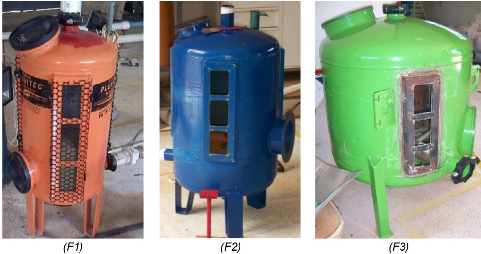
Fig 3. Commercial sand filters models evaluated, with detail of the tempered glass side panels installed.
