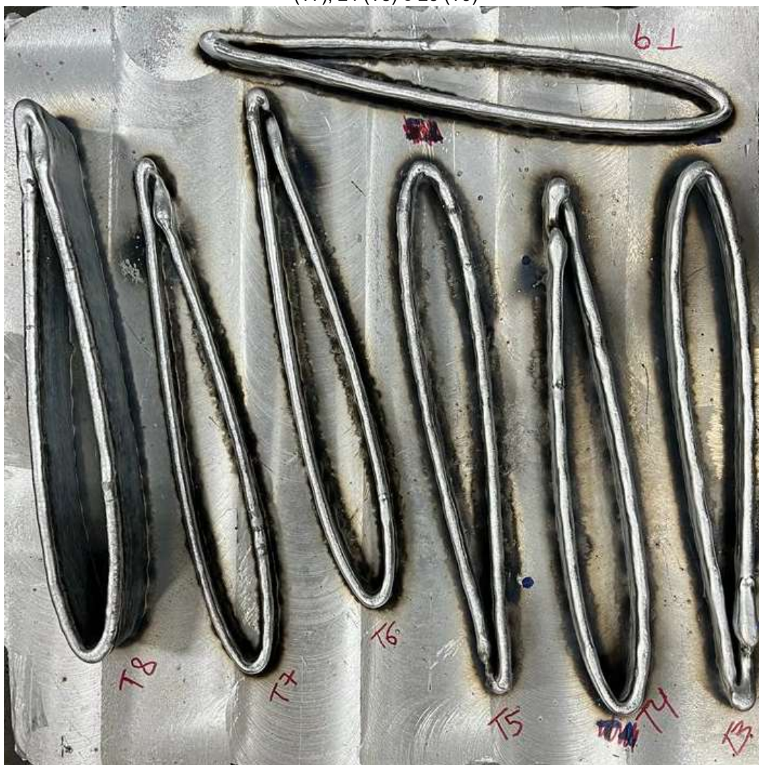
Figura 4.16 – Aspecto visual superior dos aerofólios dos testes 19 (T3), 20 (T4), 21 (T5), 22 (T6), 23 (T7), 24 (T8) e 25 (T9)
