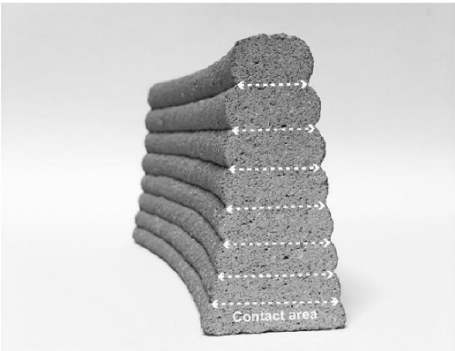
Figure 2 - Excessive deformation of the lower mortar layers after printing, showing poor printability (Chen et al. , 2020b)
