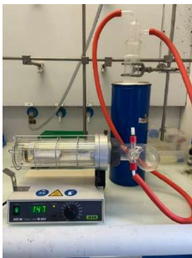
Figure 13. Dehydration of yttrium acetate tetrahydrate in a glass oven connected to a vacuum line, in the presence of P_2O_5 (Created by the author).
