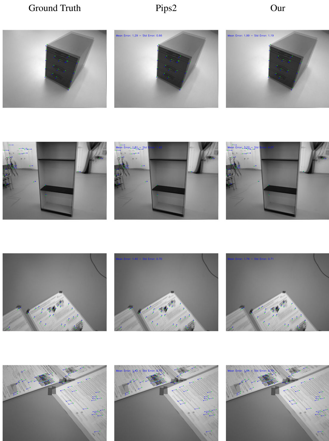
Figure 5.9: Comparison of feature tracking accuracy against the Pips2 baseline across four sequences from the TUM dataset. The mean and standard deviation of the End Point Error (EPE) are overlaid on the respective frames, illustrating the comparative performance and drift of our method relative to Pips2.
