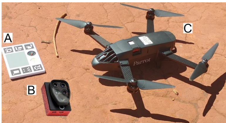
Fig. 3. A: Calibration panel that accompanies the Parrot Sequoia camera for radiometric calibration of images; B: Parrot Sequoia multispectral camera. The central wavelengths of the bands are 550 nm (40 nm) green, 660 nm (40 nm) red, 735 nm (10 nm) red edge, and 790 nm (40 nm) NIR; C: Bluegrass UAV, from Sensefly company.
