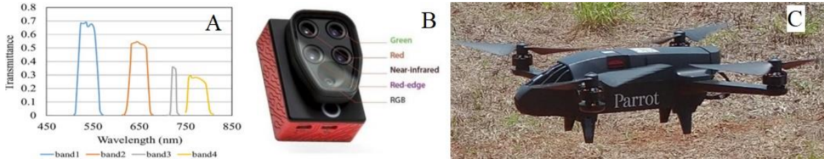
Fig. 3 A: Parrot Sequoia sensor spectral response function. The central wavelengths of the bands are 550 nm (40 nm) Green, 660 nm (40 nm) Red, 735 nm (10 nm) Red-Edge, and 790 nm (40 nm) NIR, adapted from Deng et al., (2018); B: Parrot Sequoia multispectral camera; C: Bluegrass UAV, from Sensefly
