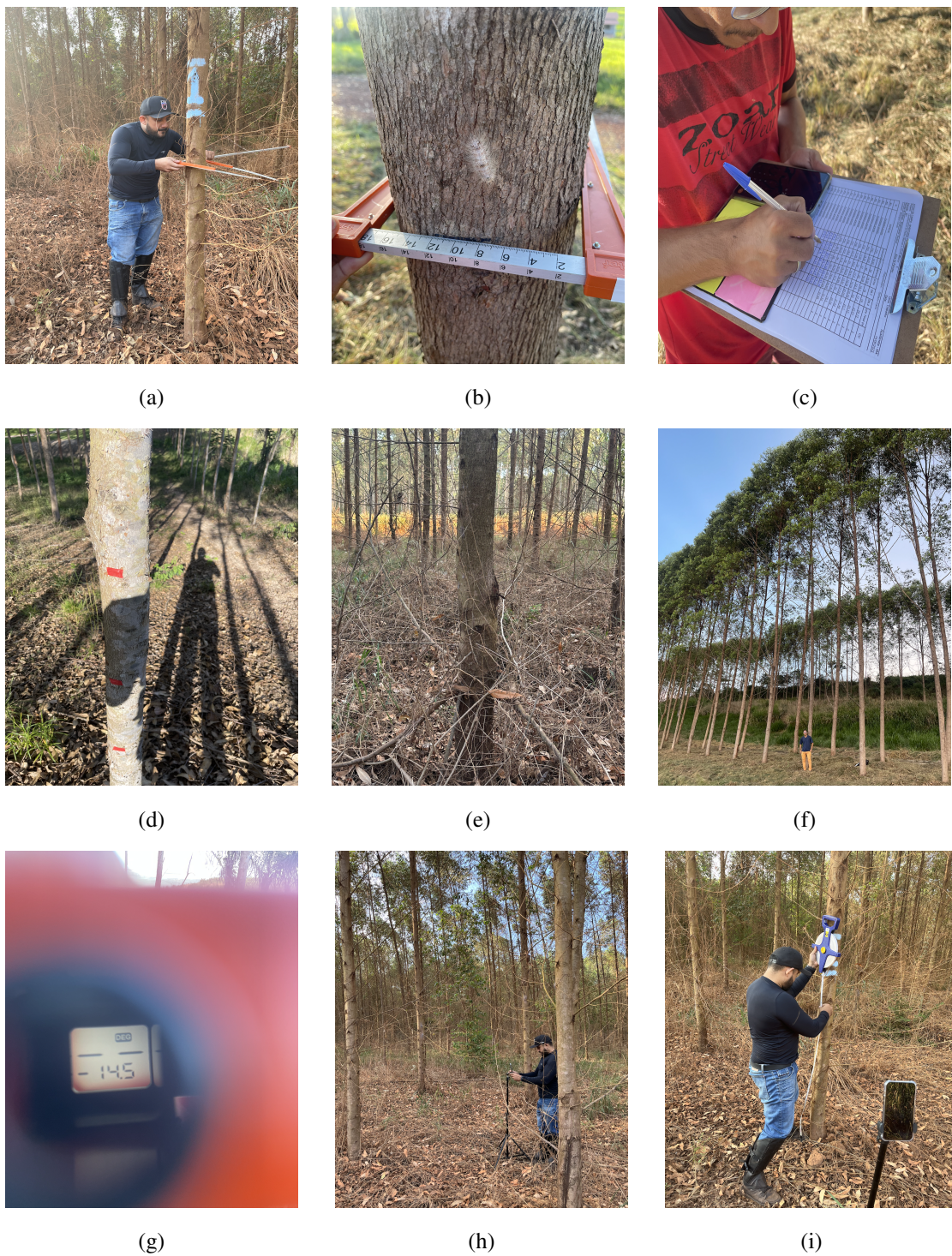
Figure 1.3: On-site data collection process. (a, b) Measuring diameter with a forestry caliper. (c) Recording field data. (d) Tree marked at the standard DBH height. (e, f) Views of the eucalyptus stand environment. (g) Measuring tree height with a digital clinometer. (h, i) Acquiring 3D data with a smartphone-based LiDAR scanner.
