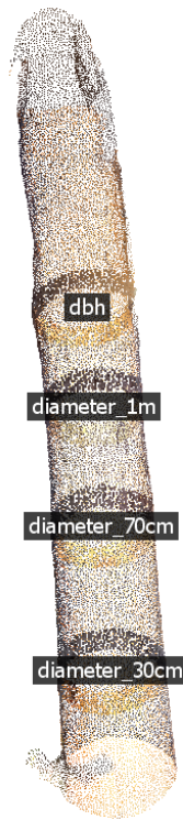
Figure 6.3: Manually annotated LiDAR point cloud of a tree stem segment, showing regions explicitly labeled for diameter measurements (DBH, 1m, 70cm, and 30cm). The remaining points on the stem segment constitute the 'stem' class, according to the annotation scheme used for training the deep learning model.
