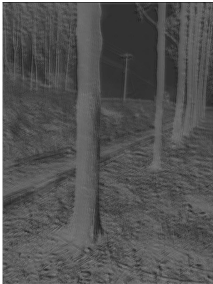
Figure 9.7: The high-resolution depth map generated by the MobileNetV2 super-resolution model, which exhibits significantly enhanced geometric detail.
