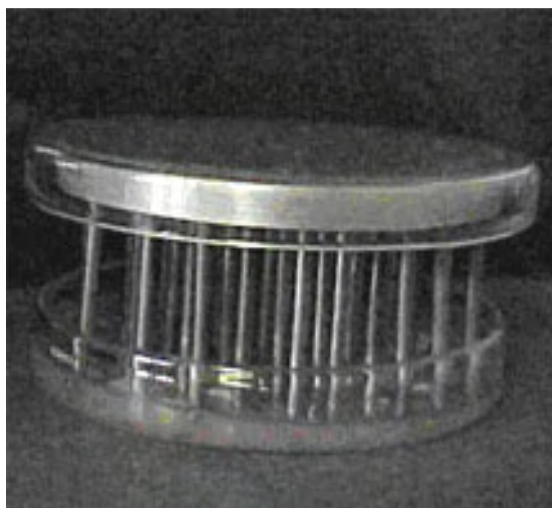
Figure 1. Formation of holes of 3 mm diameter in melted RPMI agar medium by using steel perforators in agar dilution method.
