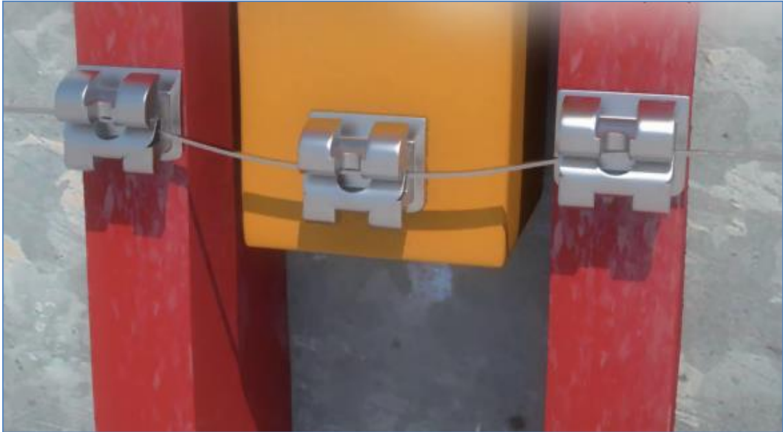
Figure 3. Three-bracket bending test.
