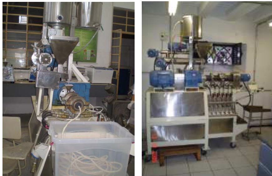
Figura 7. Extrusora INBRAMAQ, modelo RXPQ Labor 24.
