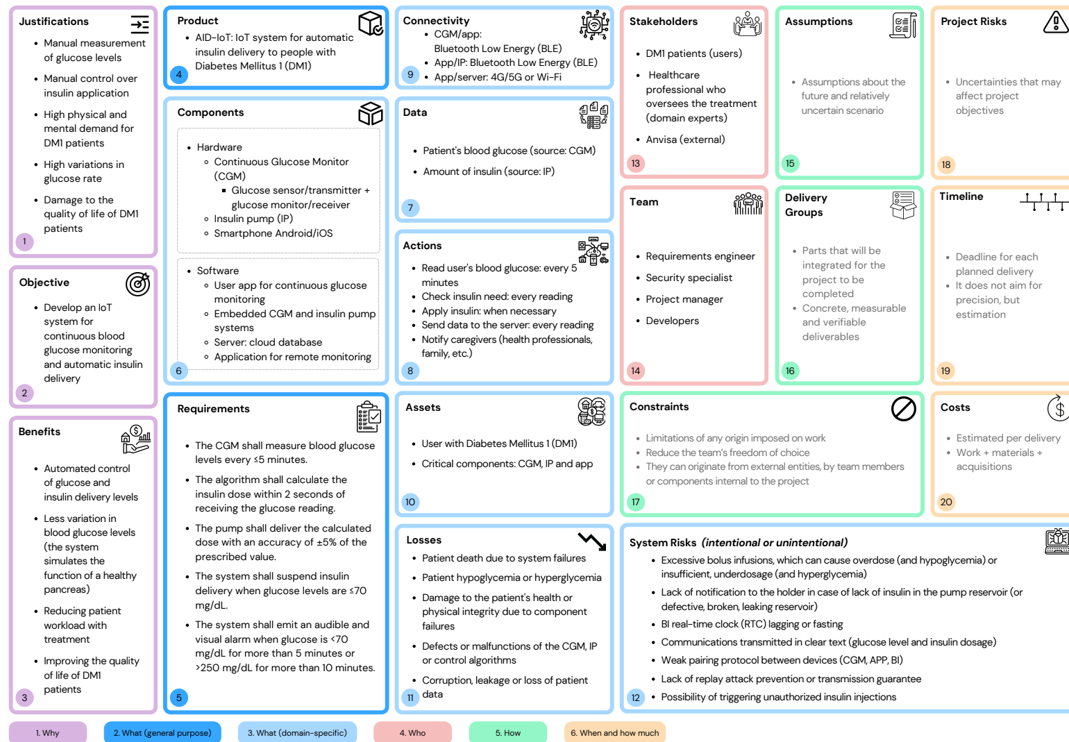
Figure 5.7: SafeSecIoT Canvas for agile project planning of an Automatic Insulin Delivery system.
