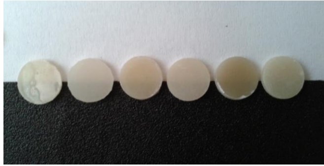
Figure 4 – Picture of the specimens of each group, in order: control groups (G1 and G4), 0.05% silver groups (G2 and G5) and 0.07% silver groups (G3 and G6). The color change caused by silver can be noticed in white and black background.
