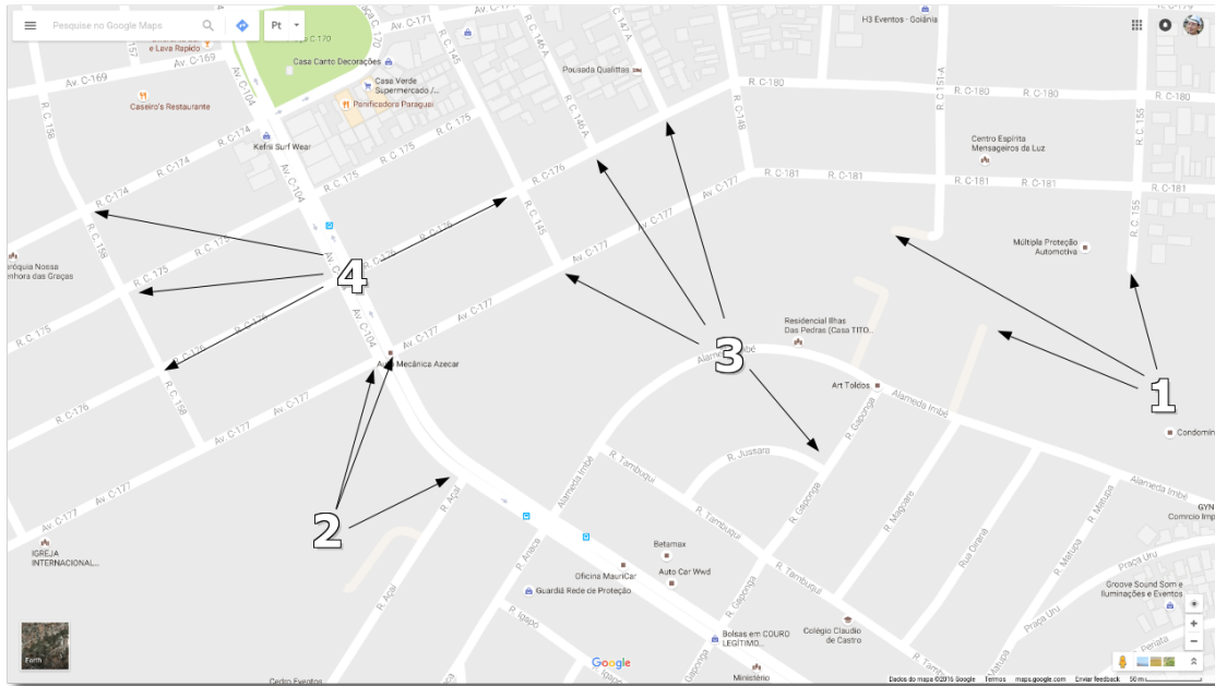
Figure 7.2: Intersections and their respective outdegrees for a small region of the city of Goiânia, Goiás, Brazil.
